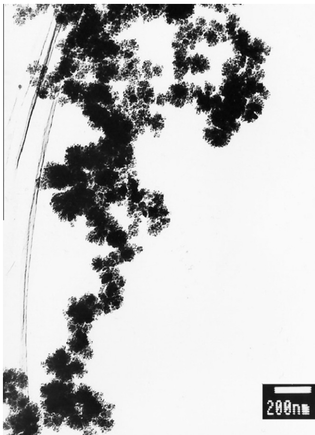
Fig. 1. Transmission electron micrograph of a typical fractal-like particle aggregate formed from a vapour mixture of Fe, Mg and Si precursors.
